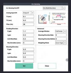
RB Series has built-in sim tracking functionality through arc sensing (current sensing). Through this function, robot can automatically track the center line of the weld while weaving and automatically adjust the height of the wire. It can be applied in a variety of ways, such as MIG/TIG welding.
